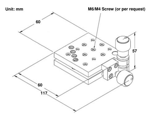
All the dimensions can be fabricated per your request, and the same with the interface layout.
